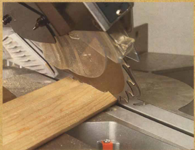
To miter crown molding with a compound-miter saw, lay the molding flat on the saw's table.
