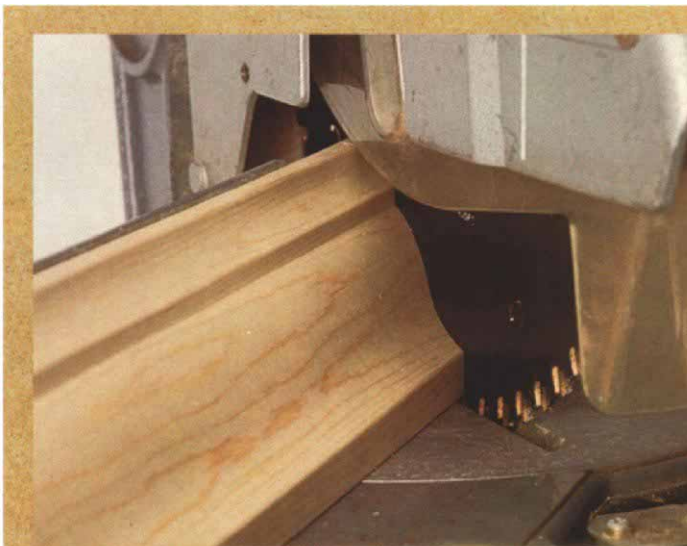
To miter crown with a standard miter saw, turn the molding upside down and set it at an angle between the fence and table.
